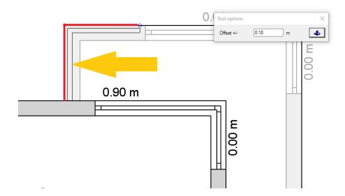
You can also set the polygon offset for existing railings any time later in our properties dialog. And as usual, you can also move the polygon points of a railing manually.
