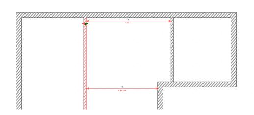
In this editing mode, you can change the direction by clicking on the respective part of the double arrow. A second click on the same part of the double arrow or on another part of the wall hides the moving dimensions and shows the usual dimension lines for the lengths again.
