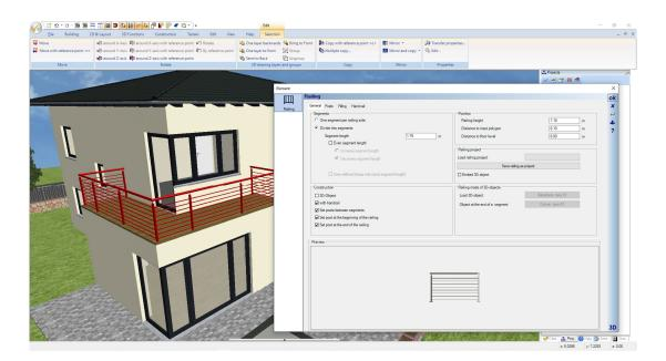
Alternatively, you can create segments of even length along the railing sides, either decrease or increase each segment.
