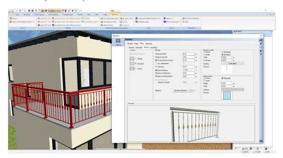
Fixed fillings, simple 3D solids with a glass material by default on it, can also be designed with other materials by dragging and dropping them from the texture or material catalog.
