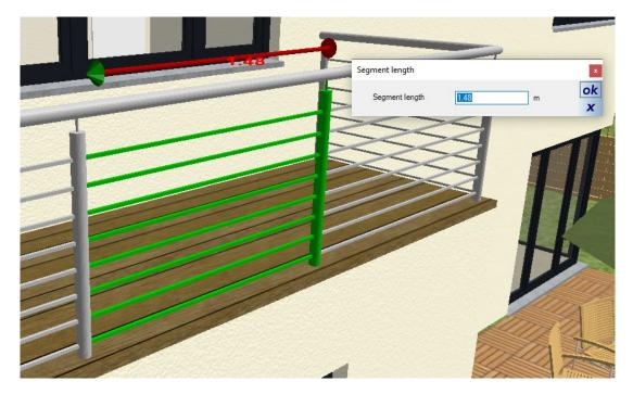
If a segment of a railing has been individually modified, the normal dividing options are disabled and the "Userdefined" checkbox shows this status.
