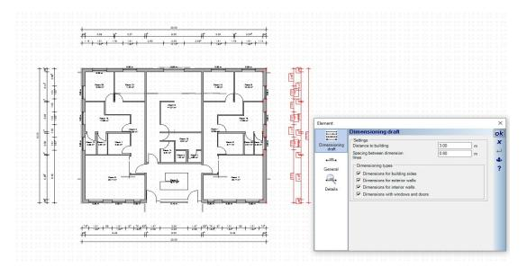
Dimensioning drafts are only generated for 2D plan views, not in section and elevation views.
