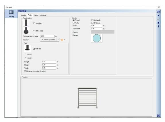
Below is a screenshot showing both mounting options. In the case an attachment at the side, it is not clear to which side the attachment must point when inserting the railing polygon.
