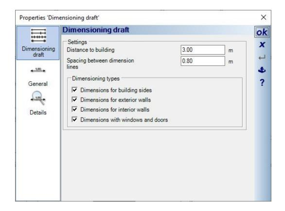
When generating the automatic dimensioning draft, the current floor plan is analyzed and the required dimension lines are generated depending on the floor plan layout. Regardless of the settings in our dialog, it can happen that you do not receive the four activated dimension lines, but only those that make sense. If there are no windows and doors on one side of the building and no offset in the facade, the software creates, for example, only two dimension lines instead of the predefined four.
