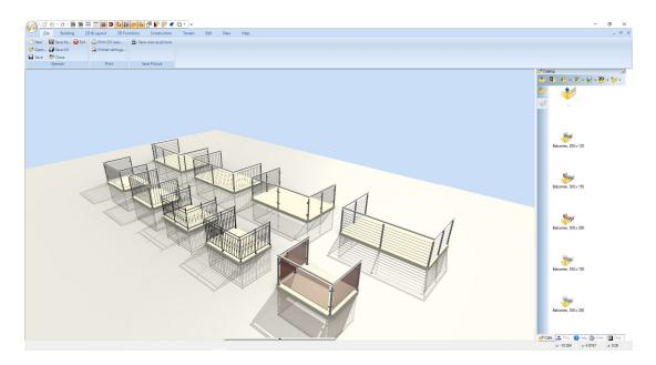
These balconies consist of three parts, two extrude solids for the floor slabs, one as a "replacement" for the ceiling and one as a covering. The railing is mounted on it.
