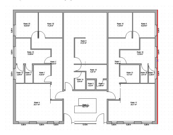
Select the wall side with a left mouse click and then move the cursor to the point where the automatic dimensioning should be inserted. So usually away from the building. At this point you will only see a cursor
