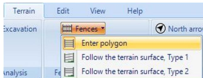
Fences are also created in segments whose length is adjustable, just like railings. At the end of each segment, i.e. where posts are typically placed, the fence determines the height of the terrain and adjusts the height accordingly. This is how the progression is created.
