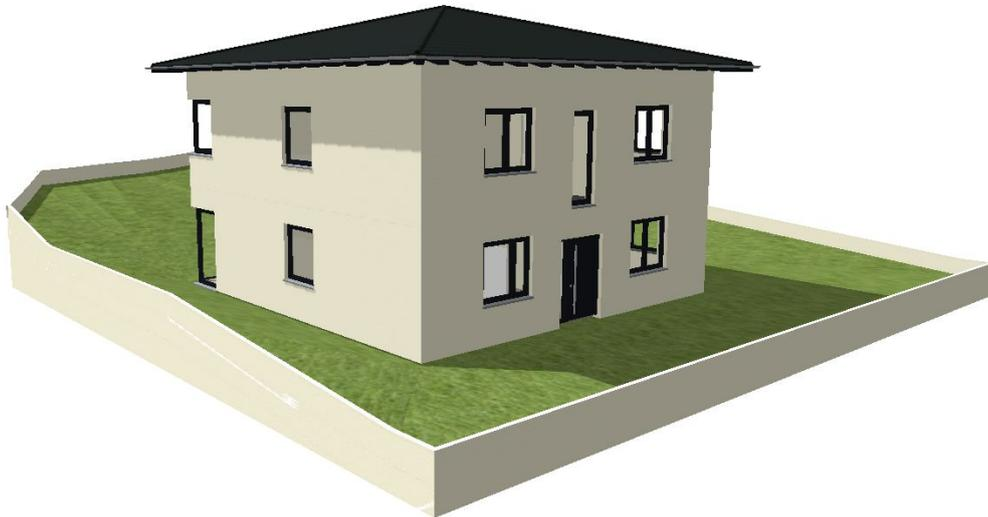
The plot forms a closed 3D solid downwards like the terrain itself. Also with the necessary depth. This prevents a basement, for example, from becoming visible below the surface of the plot.
